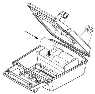
Install batteries in power pack battery adapter.
